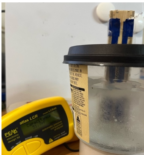
Fig. 14: To maintain an ice point, we kept ice inside the container.
